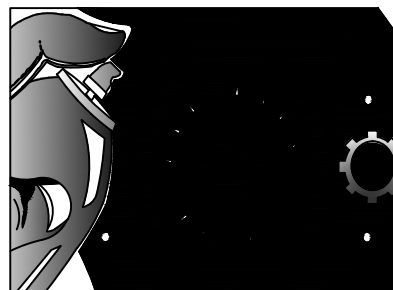
Above: For factory recommended functional testing, spray the proper test gas directly at the detector head from a distance of 12 inches for 2 seconds.
