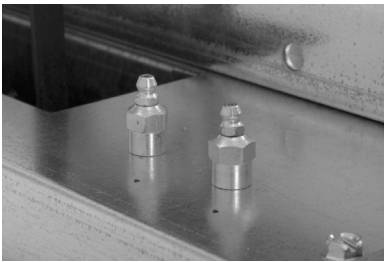
External Grease Fittings
